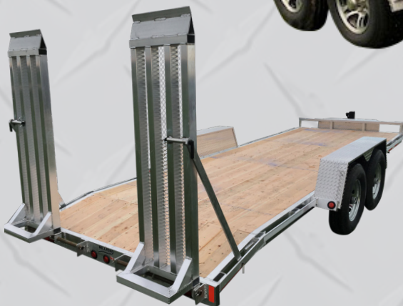
MFT2080-7 w/ A-frame tool box & rod mounted ramps
