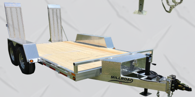
MFT2080-7 w/ A-frame tool box & rod mounted ramps
